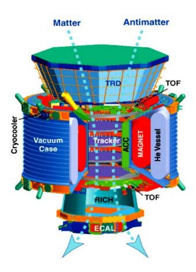
300,000 channels of electronics  $\Delta t$  = 100 ps,  $\Delta x$  = 10 $\mu$
